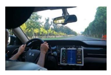
ASTRI and Huawei demonstrated the V2X applications using Huawei's world-first dual-mode C-V2X roadside device RSU, supported by ASTRI's C-V2X software system and algorithms. Under the test case, vehicles and the infrastructure leveraged C-V2X Uu and PC5 Communications channel to broadcast vehicular movement and traffic status information to cars made by FAW and other manufacturers.
