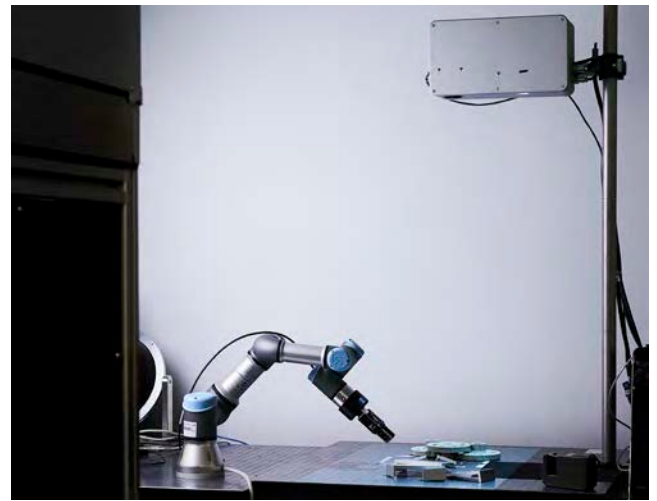
3D vision system with machine deep learning based algorithms for defect inspection and 3D random bin picking technology 三維視覺系統兼具備機器深度學習程式計算，可用於瑕疵檢測以及工業機器人的3D隨機堆疊取放技術
