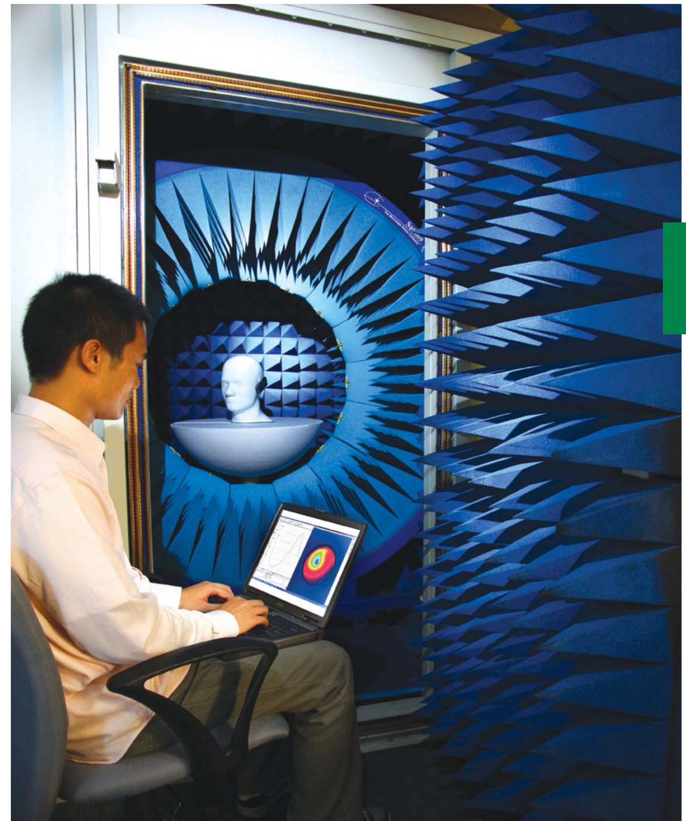
Measuring the 3D radiation pattern of a phone next to a phantom head
